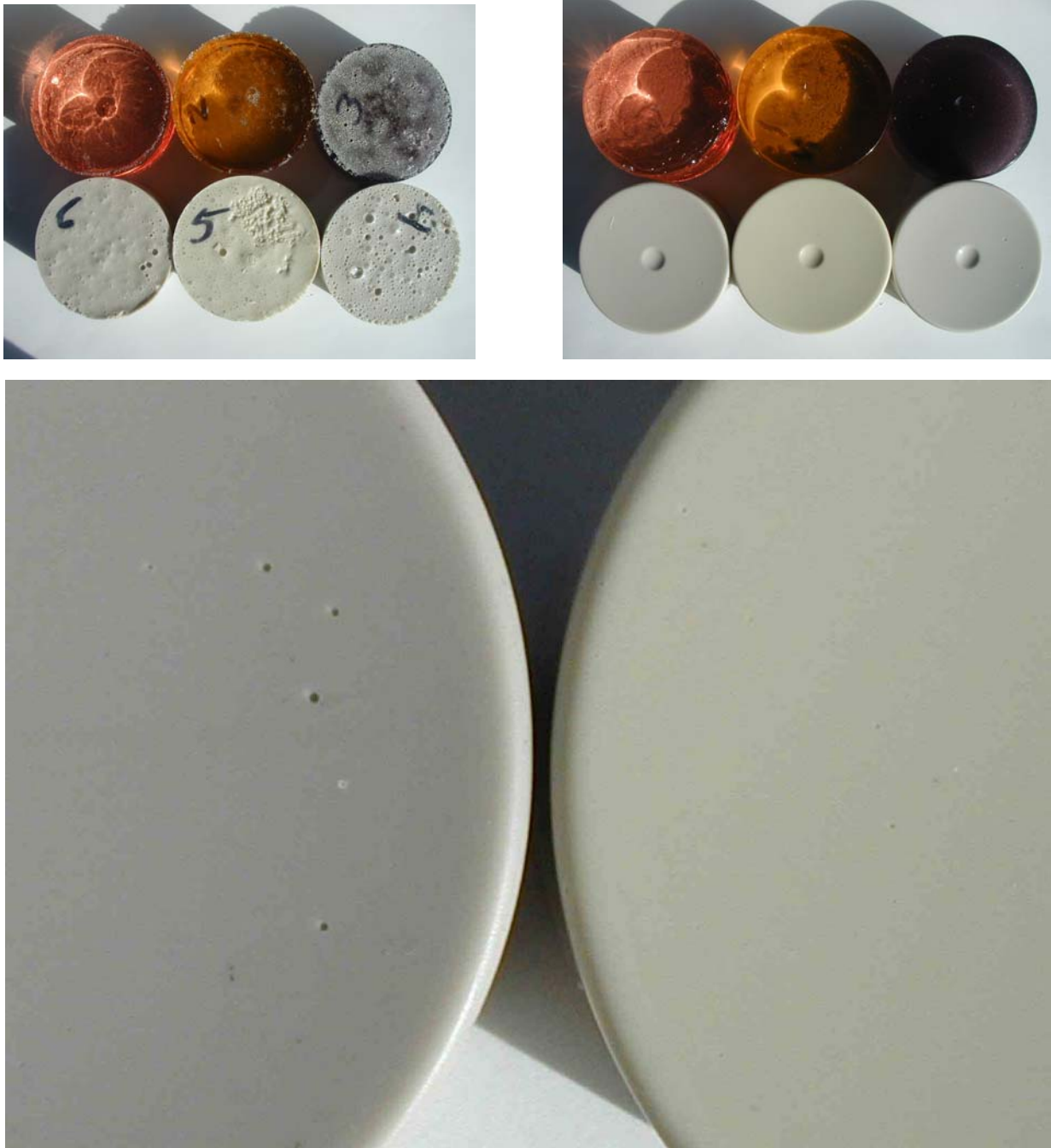
Figure 7 – Photos [(upper-left = top-side of poured in mold) and (upper-right = bottom-side of poured in mold)] show the results of the cast polyester formulations in Table 4 for Unfilled (Casting 1 = Control; Casting 2 = CP-03; and Casting 3 = CP-03 + 0.4 parts of 6% Co Naphthenate) and 60% CaCO 3 Filled (Casting 6 = Control; Casting 5 = CP-03; and Casting 4 = CP-03 + 0.4 parts of 6% Co Naphthenate). The larger lower photo is a close-up of the bottom-side of castings 6 (left – Control with pinholes) and 5 (right – CP-03 without pinholes) demonstrating the use of CP-03 eliminates pinholes.
