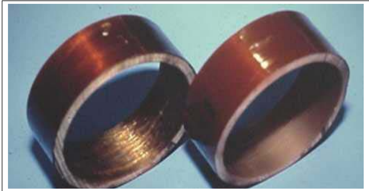
Figure 4 – The silane-sized fiberglass wound epoxy pipe on the left without titanate shows fiberglass while the pipe with 0.2 phr Ken-React added to the resin with the same fiberglass cause complete wet-out and “disappearance” of the fiber with a subsequent significant increase in resistance to hydrostatic pressure.
