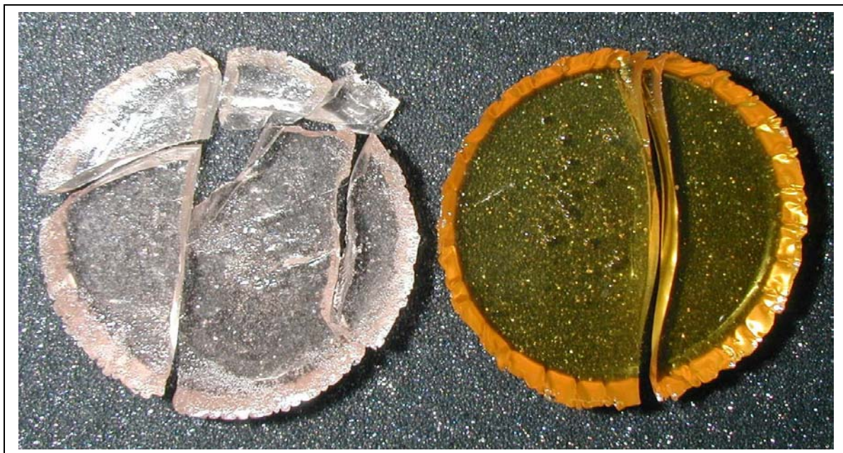
Figure 1 – Drop Impact of Polyester Castings (2¼” x ¼” discs) from 6’ Height – Ashland Polaris® MR 20000 SHV Polyester Resin (98.75 parts) cured with Norox® MEKP-925 (1.25 parts) and no Ken-React [left disc] and with Ken-React CP-03 (0.375 parts) [right disc]. The control disc was dropped once and shattered. The Ken-React CP-03 disc bounced on the 1 st drop and broke on the 2 nd drop.
